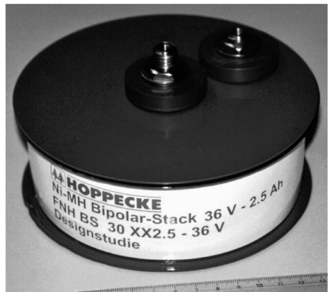
Fig. 9. Bipolar stack design.
